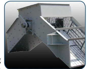
Liners Available: 550 Brinell, AR400, Tri-Braze, Stainless Steel, Tivar 88 (1/4" up to 1" thickness)
