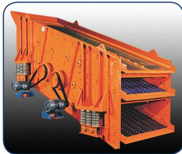
Circular motion inclined screens typically lend themselves to scalping operations. The circular motion causes the material to roll down the deck. This helps reduce "plugging" of the near size material in the openings. Elliptical motion inclined screens operate in much the same way as the circular motion version. Depending on drive placement, this screen can speed up the travel rate on the feed end and slow it down on the discharge end.
