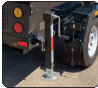
Four Manual Trailer Jacks for Unit Stabilization
