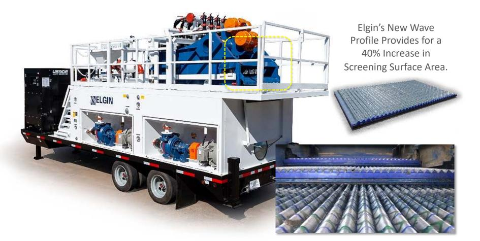
The KT-600X Deploys a Brand New Pre-Tensioned Screen Panel that Includes a Wave Profile.
