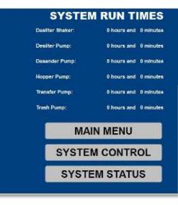
Run Time Counters Will Preemptively Notify Operators of Greasing and Maintenance Schedules. Detailed Event Logs Will Track Fault Conditions and Maintain Detail Records of the Units Operation.
