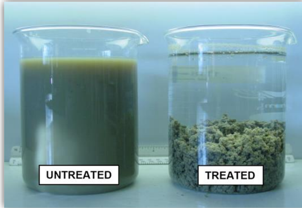
A “Chunky” Sinking Floc Tends to Provide the Best Indication of a Shear-Stable Floc
