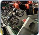
Fitted with (6) 2.5HP Hi-G linear motion vibrator motors.
