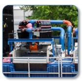
Includes forty (40) 4", ceramic-lined desilters with screen savers & valve isolation.
