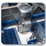
Two 5HP top-mounted agitators with gear-boxes are coupled with a series of mixing guns.
