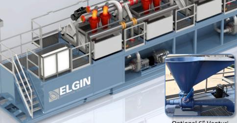
Optional 6" Venturi Polymer Mixing Hopper.
