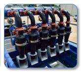
Six 4" desilter hydrocyclones, with screen savers and valve isolation.
