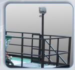
Two sets of retracting deck lights fully illuminate the working deck of the entire system.
