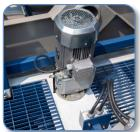
Three 5HP topmounted agitators with gear-boxes are coupled with a series of mud guns.
