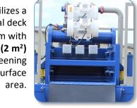
Fitted with (2) 10 HP 2x3 118 Series selfpriming closedcoupled pumps.
