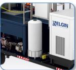
Onboard pressure washer with isolated polyurethane high-capacity water tank.
