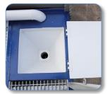
1,000 gallon partitioned tank with integrated venturi mixing hopper.
