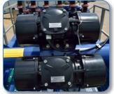
Fitted with two 2.0 HP linear motion vibrator shaker motors.
