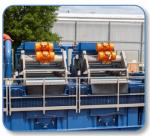
Dual Hyper-G dual-deck shakers, fitted with overhead "rock boxes".
