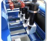
Eight 4" desilter hydrocyclones, with screen savers and valve isolation.
