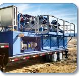
6,000 gallon, triple axel mounted tank with venturi mixing hopper.
