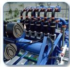
Utilizes a dual-deck shaker with 38 ft<sup>2</sup> (3.5 m<sup>2</sup>) of screening surface area.
