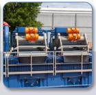
Six (6) six-Panel Dual-Deck Linear Motion Shakers with **340** ft<sup>2</sup> (**31.6m<sup>2</sup>**) of surface area.
