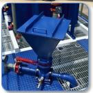
2,350 gallon partitioned tank with venturi mixing hopper.
