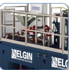
Valve-isolated 4" venturi mixing hopper with jet shear manifold.
