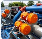
Dual 6-panel dual-deck linear motion shakers with **112** ft<sup>2</sup> (**10.4m**<sup>2</sup>) of surface area.
