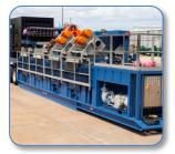
9,000 gallon triplepartitioned tank with continuous recirculation cleaning system.
