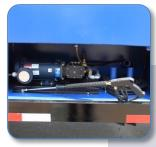
Optional onboard high-pressure washer for system cleaning.
