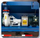
Fitted with (3) independent 40/40/40 HP 6x5 250 series centrifugal pumps.
