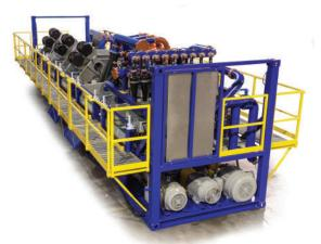
KEMTRON 1500 Pro™ skid with three (3) dual-deck scalping shakers, single-deck desander mud cleaner. and single-deck desilter mud cleaner.
