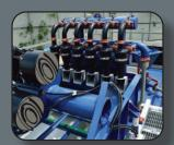
**Linear Motion Shaker** Double-deck, four panel linear motion shaker with 2.0 hp vibrator motors.
