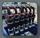
**Hydrocyclones** Six 4" desilter hydrocyclones for secondary sand and silt removal.
