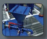
**Additives Hopper** 3" solids hopper with Venturi nozzel.
