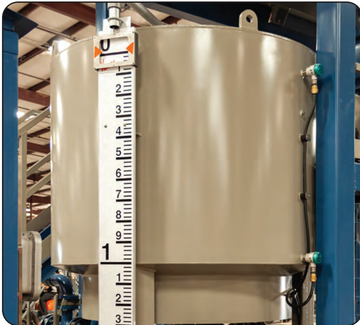
Elgin's Sophisticated Centrate Collection System Provides Operators Onboard Transfer Pump, Exterior Level Gauge, and High/Low Level Tank Sensors
