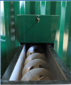
Exterior Screw Conveyor for Solids Discharge
