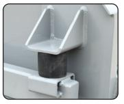
loads. This results in consistent vibration isolation with variable loading. Due to the rubber construction, Marsh Mellow<sup>™</sup> springs do not bottom-out like coil springs. Bottoming-out under overload or surge load sends a large amount of stress to all of the machine's components.
