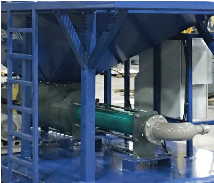
Solids Auger Integrated Progressive Cavity VFD Driven Pump with Run Dry Thermal Protection and Onboard Spray Bar Pump.
