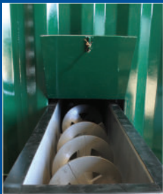
Exterior Screw Conveyor for Solids Discharge
