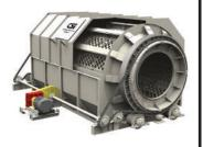
Desirable sized material passes through screen perforations and into a product hopper. Undesirable material traverses through the breaker and out the discharge end for disposal. The simple design of a rotary breaker requires little maintenance, making it economical & easy to operate.
