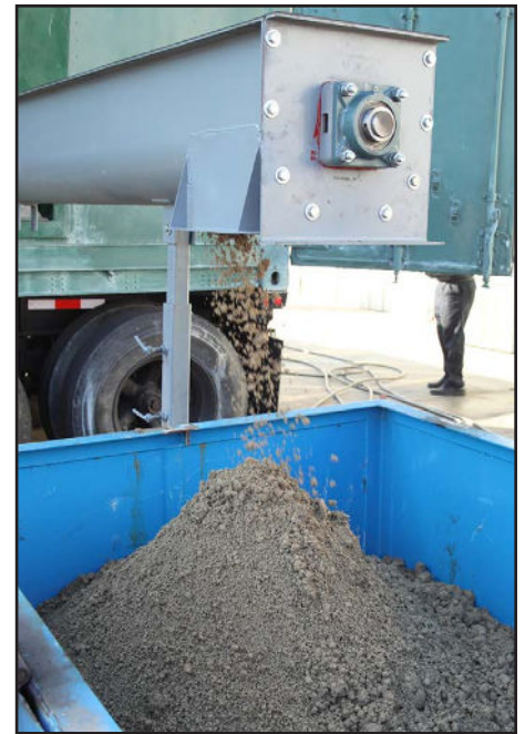
Figure 13 – Dry Solids Discharge from a Elgin DFD System
