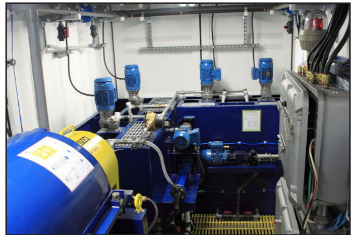
Figure 9a and 9b – Elgin’s DFD Polymer Injection and Conditioning Manifolds
