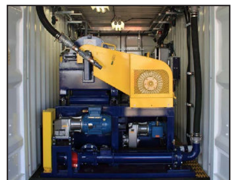
Figure 8 – 20’ DFD Systems Fed Via Progressive Cavity or Rotor Lobe Pumps
