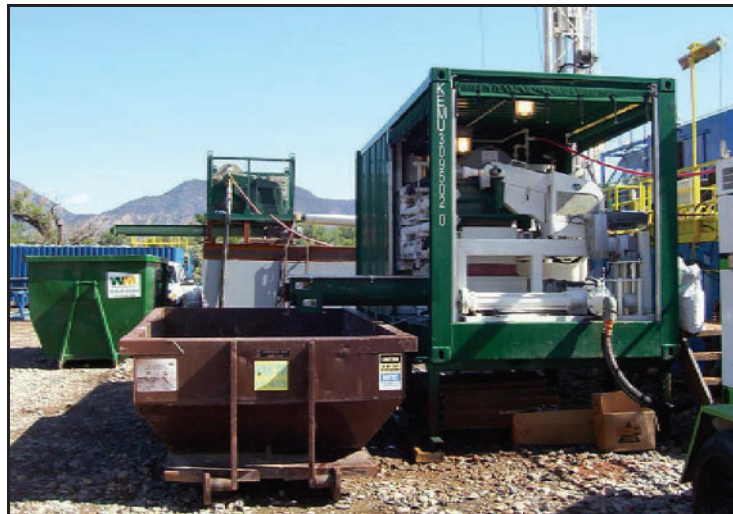
Figure 4 – Elgin's DFD System Can Eliminate the Need for Reserve Pits
