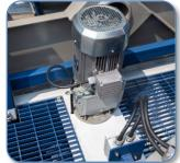
Two 5HP top-mounted agitators with gearboxes are coupled with a series of mixing guns.
