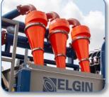
Fitted with three (3) independent 75HP 6x8x14 250 Series slurry pumps. Includes up to fifteen (15) 10" desanders , therefore able to manage up to 4,000 gpm. Can be fitted with a 200KW+ Generator Package.
