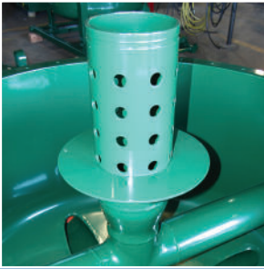
Perforated fluid inlet pipe for equal distribution of fluid across weirs.
