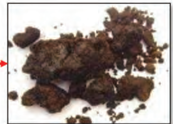
BEFORE – Drill cuttings prior to feeding through a VCD.
