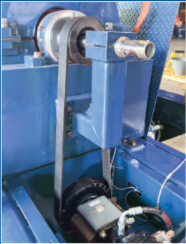
Main drive V-belt inline position ensures continuous performance and tension.
