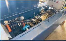
Motor, Hydraulic Components, and fluid tank engineered into base structure.
