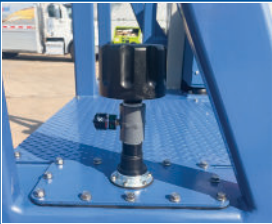
Dedicated breather unit prevents dust from entering fluid tank.
