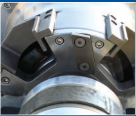
Four, "wide-mouth" tungsten carbide discharge ports and plows
