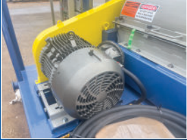
50 HP Motor connected to base of the skid structure.
